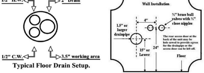
Scenario #1 = typical floor setup for the drain and water lines. Scenario #2 = typical wall setup and dimensions for the drain & water lines.
