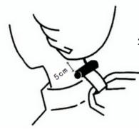
1.Set height by adjusting the supporting tube to place the rubber piece behind client's neck.
