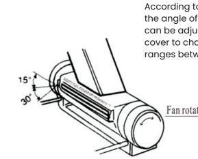
According to the length of client's hair, the angle of the fan behind the neck can be adjusted. Rotate the adjusting cover to change the angel, which ranges between 15 to 30 degrees.
