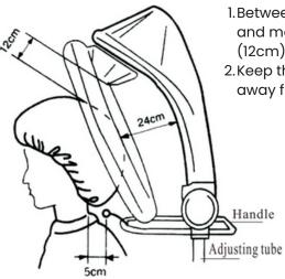
1. Between the top point of client's head and machine's rotation center, a 5" (12cm) distance should be reserved 2.Keep the rubber piece about 2" (5cm) away from the back of client's neck.
