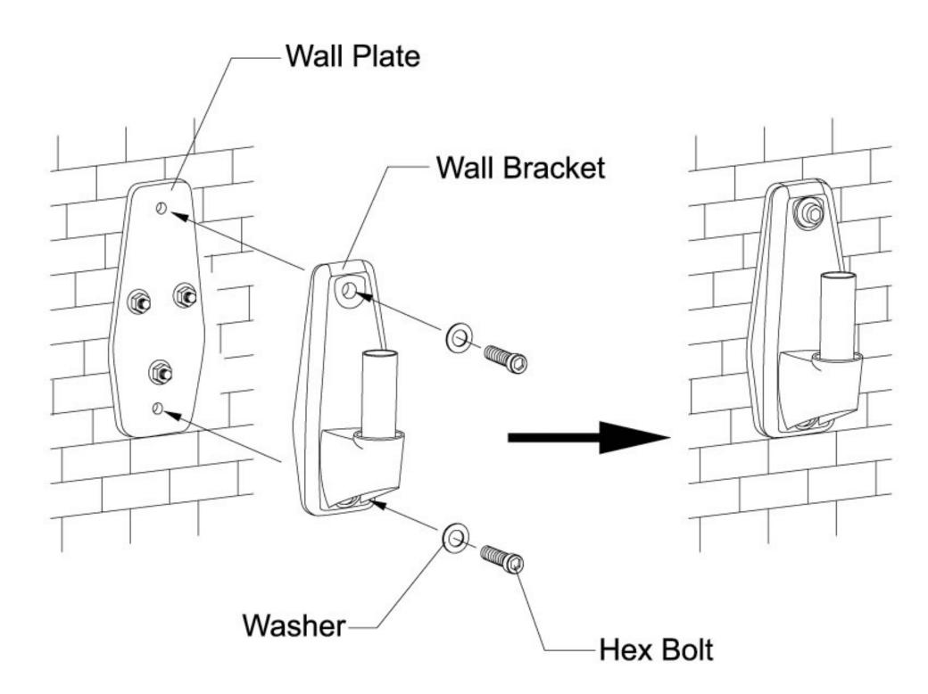
CAUTION: As the wall plate and the wall bracket are subject to a large pressure, make sure that the wall plate is installed correctly and firmly.
