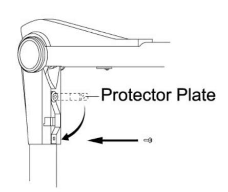
3-5 Two persons hold up the machine head and the arm assembly at the same time, then install on the wall.
