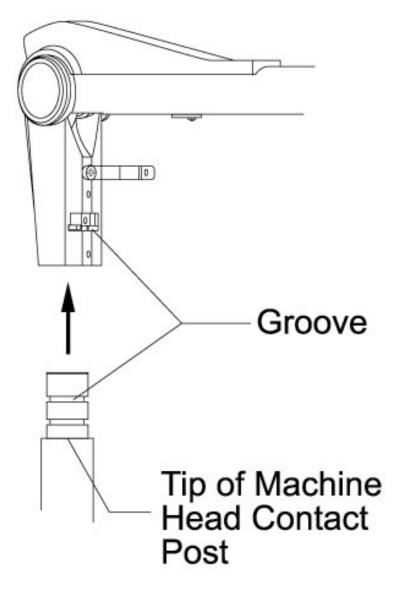
3-3 Reinstall back the hook lock to the groove and then tighten the screw firmly.
