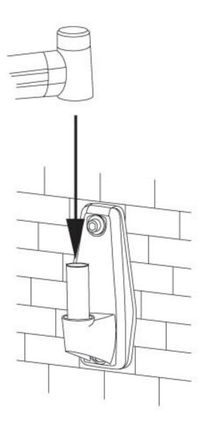
3-6 Remove the stopper, otherwise it will damage the arm assembly!
