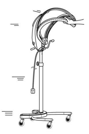
Do not move or lift PHANTOM by grabing circular heater with hand. This will damage
