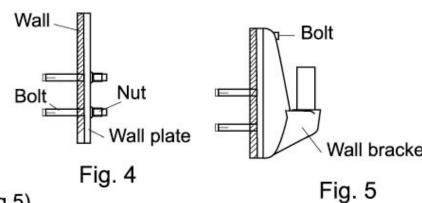
CAUTION! As wall plate and wall bracket are subject to a large load, make sure that the wall plate is installed correctly and firmly.
