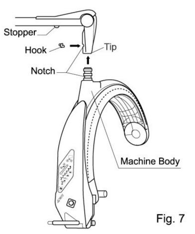
**Note 1:** Please make sure to insert the machine head contact post firmly. The tip of the arm assembly must be vertical adown. You may also turn the tip of the arm assembly left or right slightly and press the tip of the arm assembly slightly.
