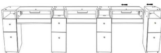
Install Bolts from the inner side flap of the two side cabinet tables
