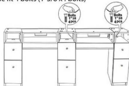
Step 4: Installing middle section
