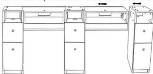
Install Bolts from the inner side flap of the two side cabinet tables
