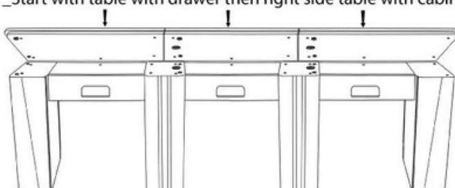
Install Bolts from the inner side flap of the two side cabinet tables
