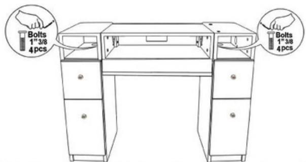
Step 3: Installing left side table
